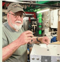
Gary WØMNA opens a repeater for visual inspection and cleaning.
